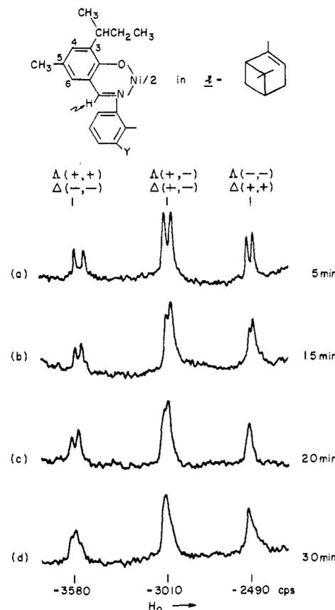
Figure 1. Pmr spectra (60 Mc,  $\sim 30^\circ$ ) of the complete isomeric mixture of Ni(3*s*Bu,5Me-sal)<sub>2</sub>bp (Y = H) in  $-47.1^\circ$   $\alpha$ -pinene illustrating the time dependence of the solvent-induced splittings of the azomethine proton signals. Intensities of components of each pair were shown to be equal by alternation of field-sweep direction. Frequencies (cps) are the chemical shifts relative to TMS.
